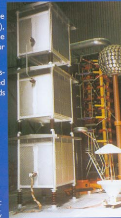
Lightning impulse on a filter resistor. HVDC Continuous current link between Denmark and Germany
