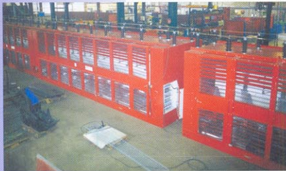
Load bank 25 MW - 5 containers of 5 MW each. (Dutch Railways)
