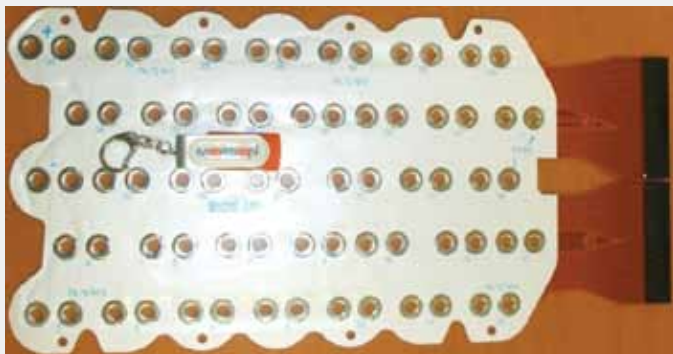
Figure 1: Mersen Monitoring Bus Bar ready to plug on lithium-ion cylindrical cells of a battery pack for electric vehicles.
