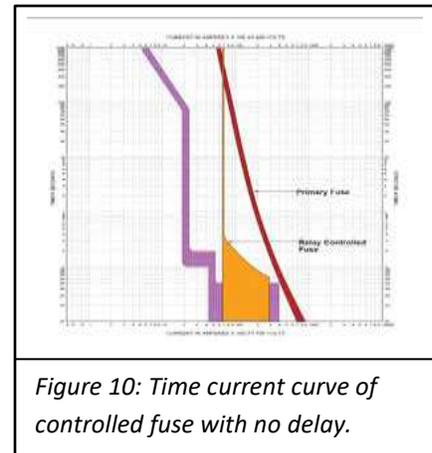
the relay and Controlled Fuse components is shown in Figure 10. The incident energy calculation for the incoming bus for both applications is reduced to 3.7 cal/cm<sup>2</sup> at 24" when in maintenance mode.
