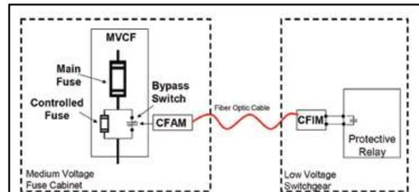
Figure 7: Controllable Fuse Diagram
