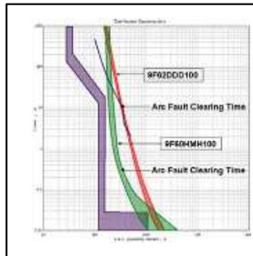
Figure 5: Time current curve for primary fuse.
