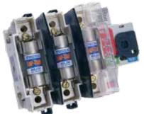
The HSJ can be used in fusible disconnect switches, providing code branch circuit protection. It can also protect power semiconductors without the need for additional protective devices.
