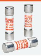
Amp-Trap® ATQ midget time-delay fuses are rated a full 500 volts AC with 42 ampere ratings from 1/10 to 30A. They are an excellent choice for supplemental protection of circuits up to 30A where the available short circuit current does not exceed 10,000A. (Not for Branch Circuit Protection).
