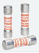
Tri-Onic® TRM time-delay midget fuses are rated 250 volts AC and are offered in ampere ratings from 1/10 to 30A. They have 12 seconds time-delay at 200% rating to provide supplemental protection of small motors, small transformers and other high inrush loads, plus many other 250 volt applications. (Not for Branch Circuit Protection).
