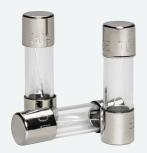
125 volt AC rated GGU fuses have midget fuse dimensions (1-1/2" long x 13/32" diameter). 20A-30A ratings have ceramic bodies, allowing use in higher ambient temperature conditions than other similar fuses. (Not for Branch Circuit Protection).
