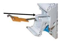
2. Slip the indicator light's to insert into the rails, being careful not to twist the contact tabs.
