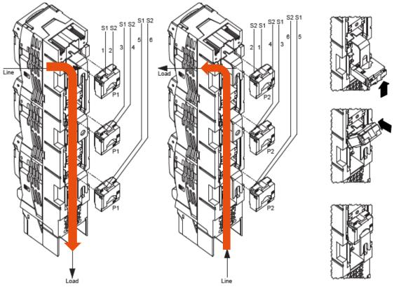
If the product is connected at the load following the "Other side load connection", 2 options :
